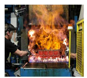
A versatile heat treatment department fully equipped for tempering, annealing, casehardening, nitro carburizing, nitride hardening and carbonitriding secures the right properties for each product.
